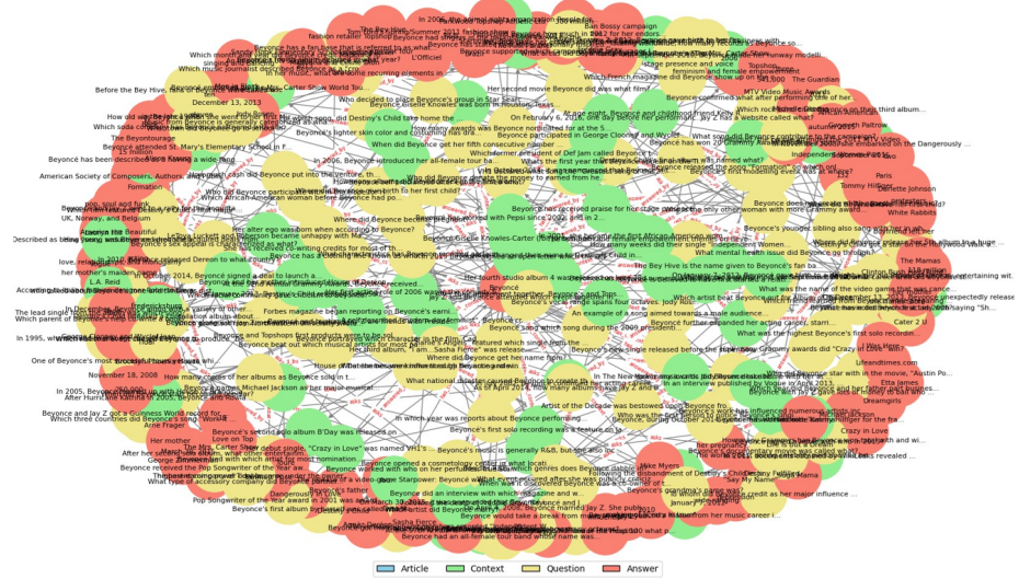
Fig. 2. Simplified Knowledge Graph constructed from SQuAD passages. Nodes are colour-coded by type: Context (yellow-green), Question (orange), and Answer (green). Edges represent semantic relations extracted via NER and RE, forming the (s, p, o) triple store queried in Stage 4.
