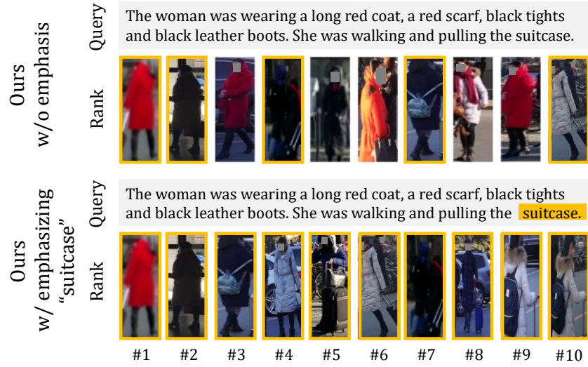
Fig. 8. Effect of emphasizing a specific phrase. Top: Retrieval results using our method without emphasis. Bottom: Retrieval results with emphasis applied. Orange frames indicate individuals actually carrying a suitcase.
