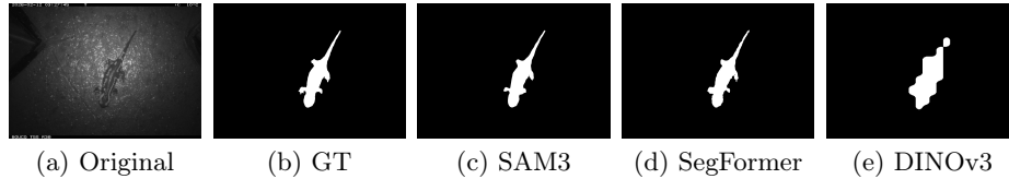
Fig. 3. Qualitative comparison of segmentation performance. The panels display (a) the original input image, (b) the ground truth mask, and the predicted masks generated by (c) SAM3, (d) SegFormer-B3, and (e) DINOv3.
