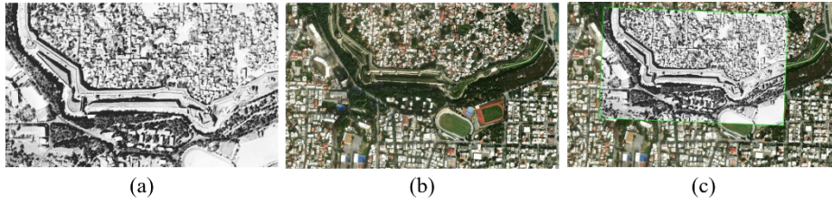
Fig. 5. Example images from the RegGR1945_2025 dataset from Rhodes Island: (a) historical aerial photograph, (b) satellite image of 2025, (c) visualization of the correct registration of the aerial photograph to the satellite image of 2025. The source of the satellite images of 2025 is the Satellites pro website [19] and of the historical aerial photographs the Hellenic Cadastre Geoportal [18].
