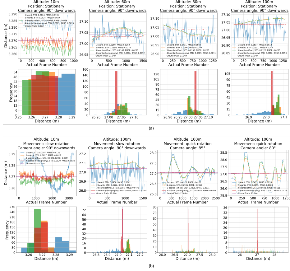
Fig. 6. The error-component-wise evaluation of 1 (marked with blue), 2 (marked with orange), 3 (marked with green), and 4 (marked with red) reference marker-based coordinate system accuracy enhancement and camera instability error mitigation in (a) stationary and in (b) dynamic use cases, from different camera positions and tilts, by ground truth target-marker distance (purple) comparison.
