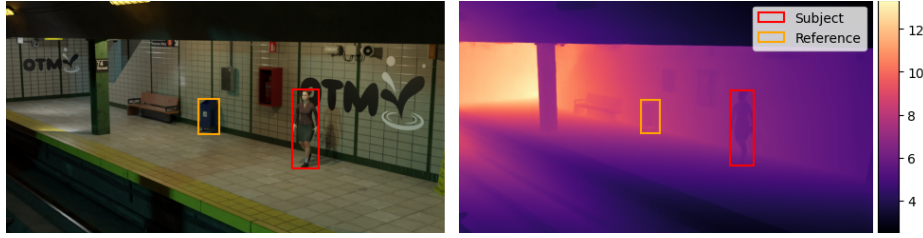
Fig. 4. Visualization of the depth estimation extraction. The left image shows a rendered RGB image from the HDA-DH-CCTV dataset with the reference object (yellow) and subject (red) bounding boxes. The corresponding image (right) visualizes the depth map (colour encodes relative scene depth) used to compute the median depth values based on the bounding box areas.
