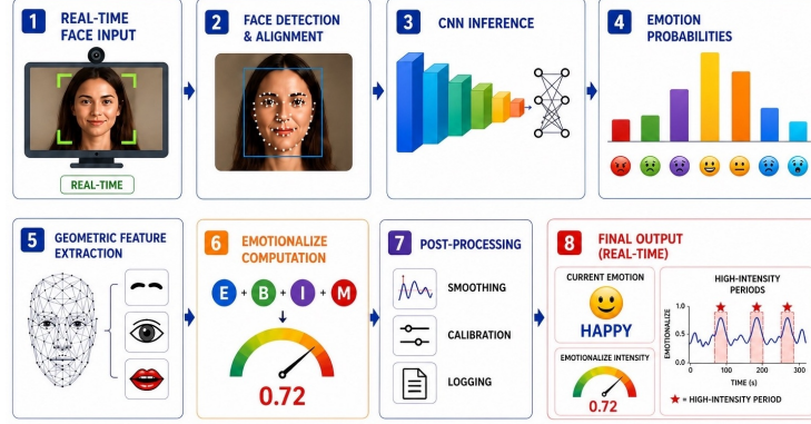
Fig. 1. The proposed real-time emotion recognition pipeline. Video frames are processed for face detection to compute the continuous Emotionalize intensity alongside the final emotion label.
