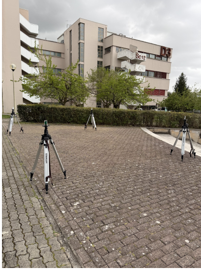
Fig. 3: Paved outdoor experimental setup with four UWB anchors placed at the corners of the 4\text{ m} \times 6\text{ m} test area.
