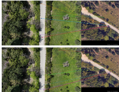
Fig. 3. Qualitative effect of pose-conditioned spatial regularization on a DJI Mavic 3 Enterprise frame. Unconstrained matching sends several road pixels to a visually similar but incorrect satellite region. Pose-conditioned matching keeps correspondences local to their predicted satellite locations, preserving the road structure for pose refinement.
